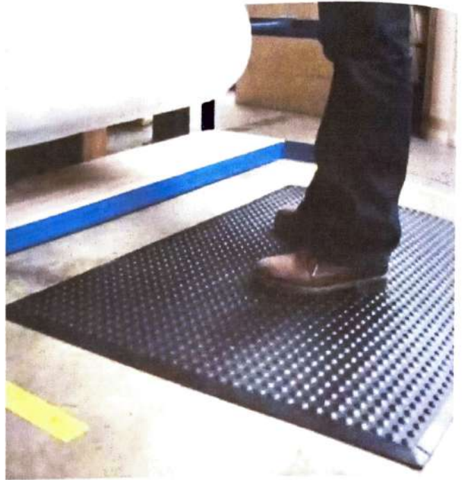
Figure 17 - Electrical safety mats
